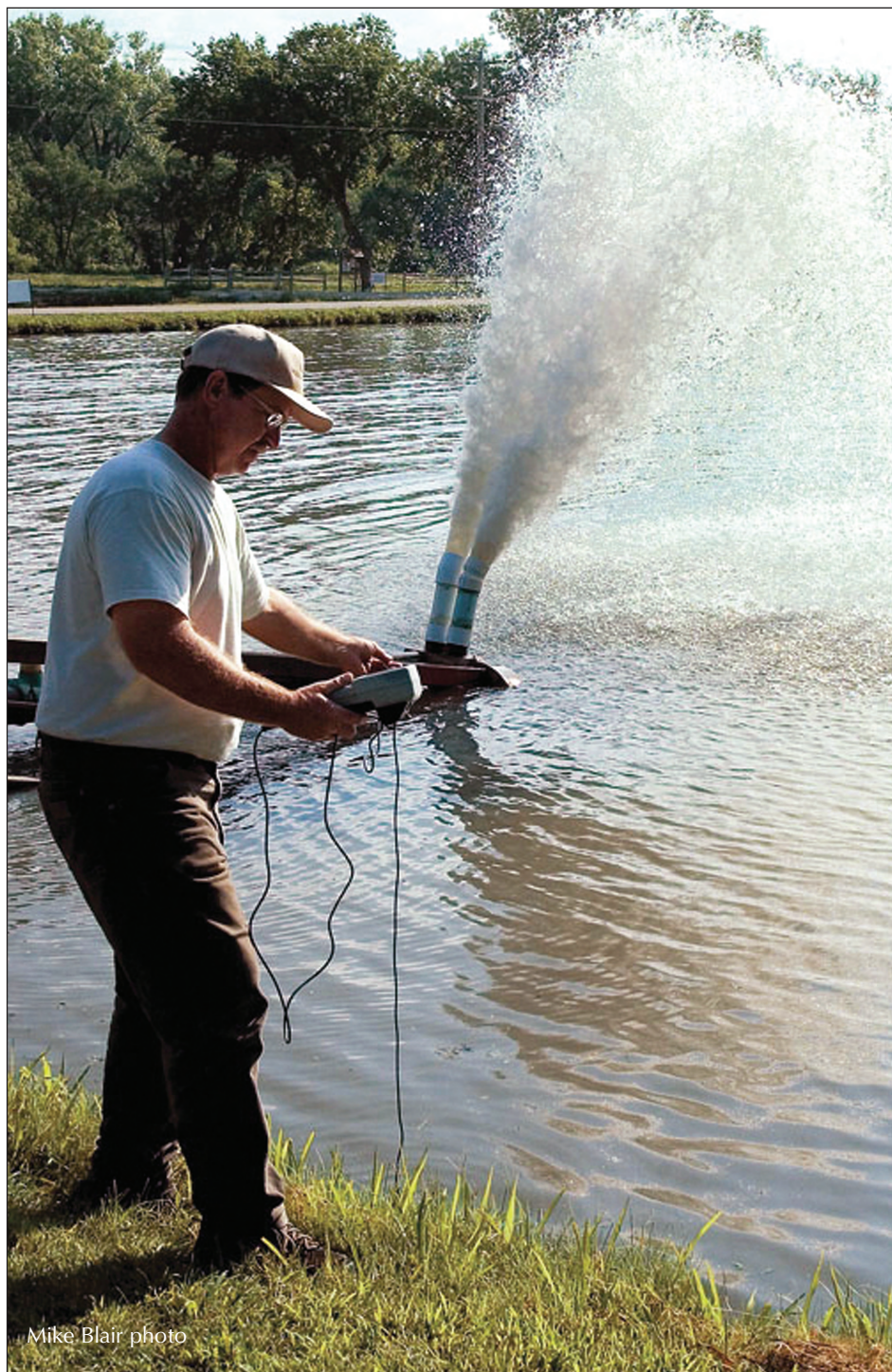
Pratt Hatchery manager Mark Kumberg reads the dissolved oxygen level of a hatchery pond while a portable aerator pumps water into the air to oxygenate it.
